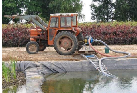
A farm tractor used to power a pump for irrigating a plot of land
