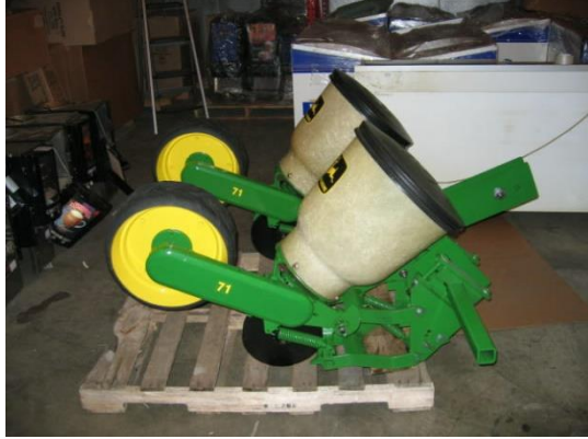
JD 71 Flexi Planter for tractors 20 to 35 horsepower
