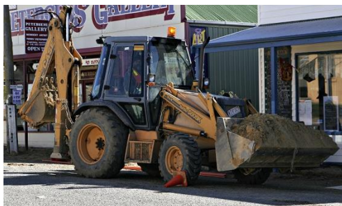
A common backhoe-loader - the backhoe is on the left, the bucket/blade on the right.
