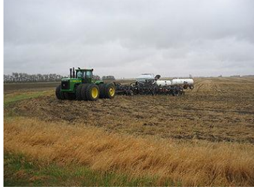
A large, modern John Deere model 9400 four-wheel drive tractor with tripled wheels and a drawbar-towed tool chain, including one-pass tillage equipment, planter and fertilizer applicator with tanks
