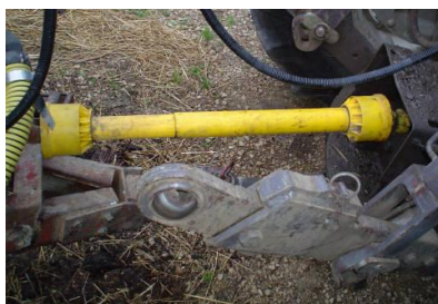
A PTO shaft connected to a tractor
