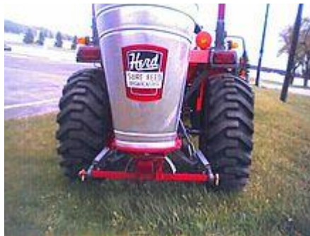
Broadcast seeder mounted to a Kubota CUT
