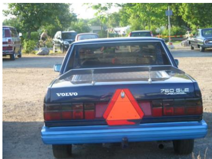
An "A tractor" based on Volvo 760 - notice the slow-vehicle triangle and the longer boot.
