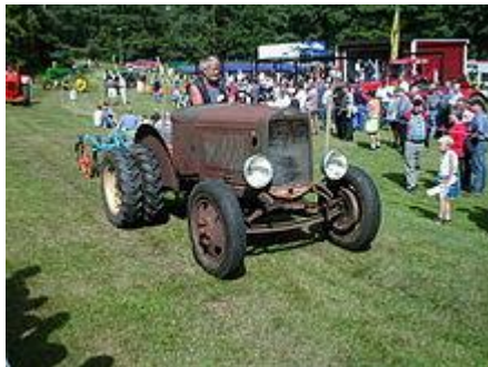
A Ford rebuilt to an EPA tractor
