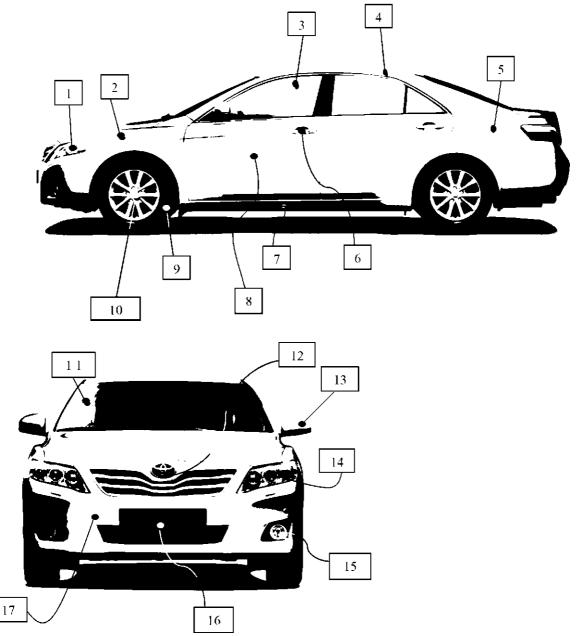
Roof - wing - indicator - fog light - side window - front bumper - number plate - logo - petrol flap - door handle - sill - door - headlight - tyre - wheel trim - front bumper - windscreen - wing mirror
