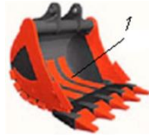
Figure 1 – View of a single-bucket hydraulic excavator bucket with reinforcing pads However, the issue of reducing the friction forces of the soil against the bottom and rear wall of the bucket remains relevant.
